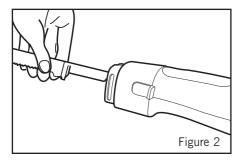
4. Insert the plug into a 230-240 volt (AC only) power outlet and ensure the cord is well away from the blades. Holding the knife with one hand, slide and press the double movement power trigger positioned under the handle to activate the motor. Releasing the switch will automatically stop the motor.
